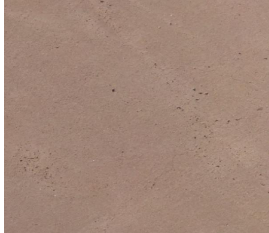
14) 70 – Scaling Low, Concrete – Section H2
